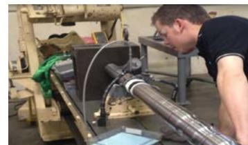
Checking for Runout
